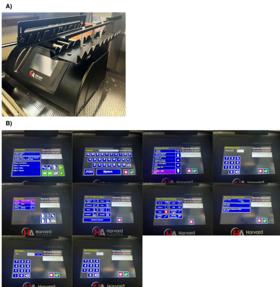
Figure 4. Automated syringe pump setup for medium replenishment and shear flow induction. (A) Programmable syringe pump equipped with an extension rack enabling simultaneous operation of multiple syringes connected to microfluidic chips. (B) Representative screen-by-screen workflow used to configure automated infusion protocols, including method creation, syringe selection, flow rate programming, pause intervals, and repeat cycles for automated medium replenishment and shear flow application. Screens are representative of the syringe pump model used in this study and may differ between manufacturers. Please click here to view a larger version of this figure.
