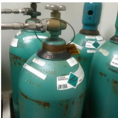
The source of inert gas used with the Pneumatic Primer can be nitrogen or argon. Ultra -high purity gases are recommended for use in this system.
