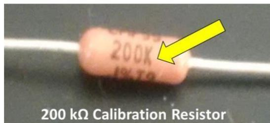
**Figure 6.** Reading the value and tolerance on the calibration test resistor. The value of the resistor is highlighted with a yellow arrow. This resistor is marked “200K”, indicating a resistor value of 200 k $\Omega$ .
