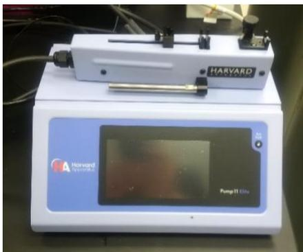
A syringe pump with an injector unit (PHD Ultra, Pump 11 Elite Nanomite is shown; Harvard Apparatus) is used to seed cells in the devices. The injector unit of the syringe pump is light enough to rest on a microscope stage for real-time viewing and imaging of cell seeding.
