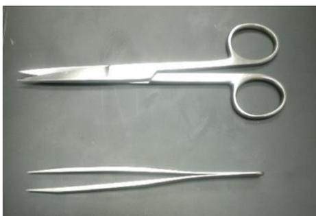
Both stainless steel forceps (ultra-fine; VWR 100494-698) and scissors (Fisher Scientific 19062530) are used to cut and insert tubing into the microfluidics devices.
