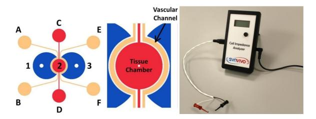
Schematic of the chip used for the SynBBB Model and SynVivo Cell Impedance Analyzer system. Vascular chambers (outer channels) are for culture of endothelial cells while the tissue chamber (central chamber) is for culture of brain tissue cells (astrocytes, pericytes, neurons). Porous architecture enables communication between the vascular and tissue cells.
