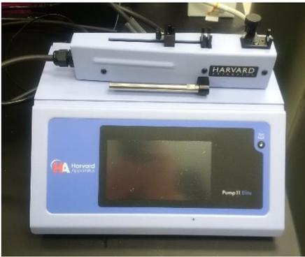
A syringe pump with an injector unit (PHD Ultra, Pump 11 Elite Nanomite is shown; Harvard Apparatus) is used to seed cells in the devices. The injector unit of the syringe pump is light enough to rest on a microscope stage for real-time viewing and imaging of cell seeding.
