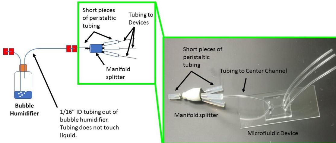
**Figure 2.** Illustration of the manifold splitter and its connection to the bubble humidifier, as well as an image of the manifold splitter connected to the center channel of a microfluidic device through tubing.
