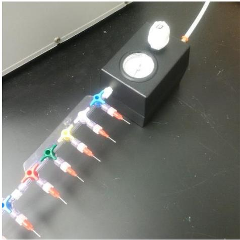
The Pneumatic Primer (SynVivo 205001) is a pressure regulator that flows inert gas at a low pressure through the SynVivo devices. A multiple port manifold (SynVivo 207001) is connected to the primer and allows perfusion of multiple microfluidics devices at once.
