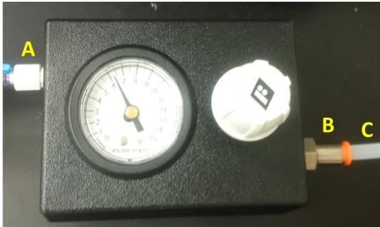
The Pneumatic Primer consists of an inlet connector that connects the microfluidics device to the pressure regulator (**Figure 1A**). On the opposite side of the pressure regulator box, a metal male connector (**Figure 1B**) will join the pressure regulator to nylon tubing containing inert gas (**Figure 1C**; use ¼ inch or 0.635 cm outer diameter; 11/64 inch or 0.436 cm inner diameter nylon tubing).
