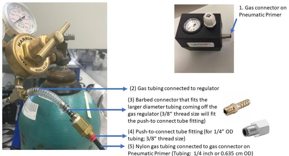
**Figure 3.** Nylon gas tubing and connectors are needed to connect the pressure regulator on the gas source to the Pneumatic Primer.
