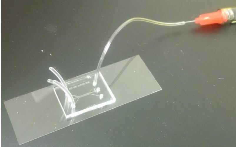
**Figure 3.** Perfusing a SynVivo linear device with PBS.
