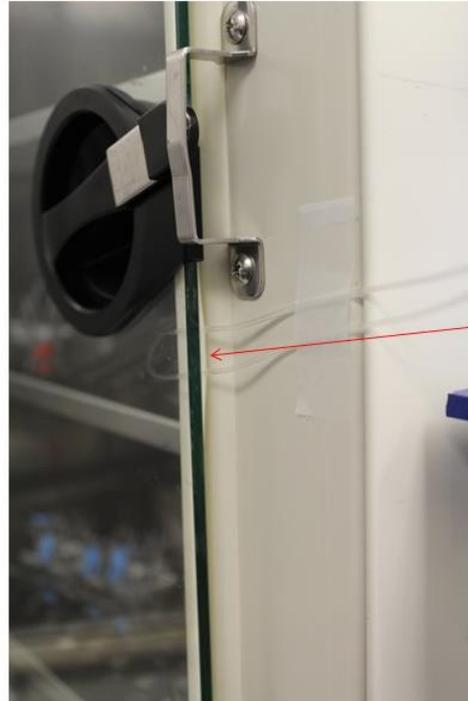
Close inner door of incubator – gasket should compress to make room for tubing
