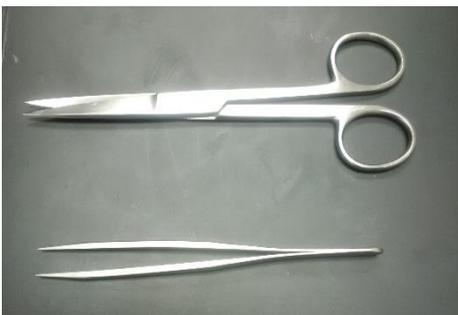
Both forceps (ultra-fine; VWR 100494-698) and stainless steel scissors (Fisher Scientific 19-062530) are used to cut and insert tubing into the microfluidics devices.
