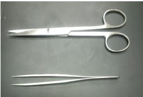
Both forceps (ultra-fine; VWR 100494-698) and stainless steel scissors (Fisher Scientific 19-062530) are used to cut and insert tubing into the microfluidics devices.
