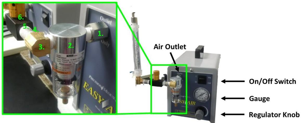
1. Steel threaded pipe fitting (McMaster-Carr 50925K541)
