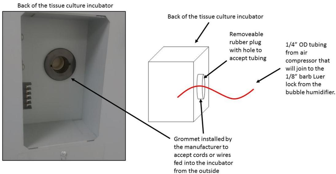
**Figure 4.** Illustration describing how to feed tubing from the air compressor into a tissue culture incubator that can accept cords or tubing from the outside through a pre-manufactured hole in the back of the incubator (access port).
