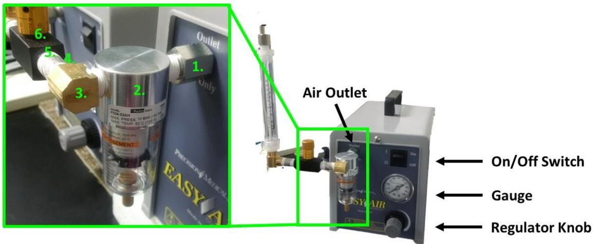
1. Steel threaded pipe fitting (McMaster-Carr 50925K541)
