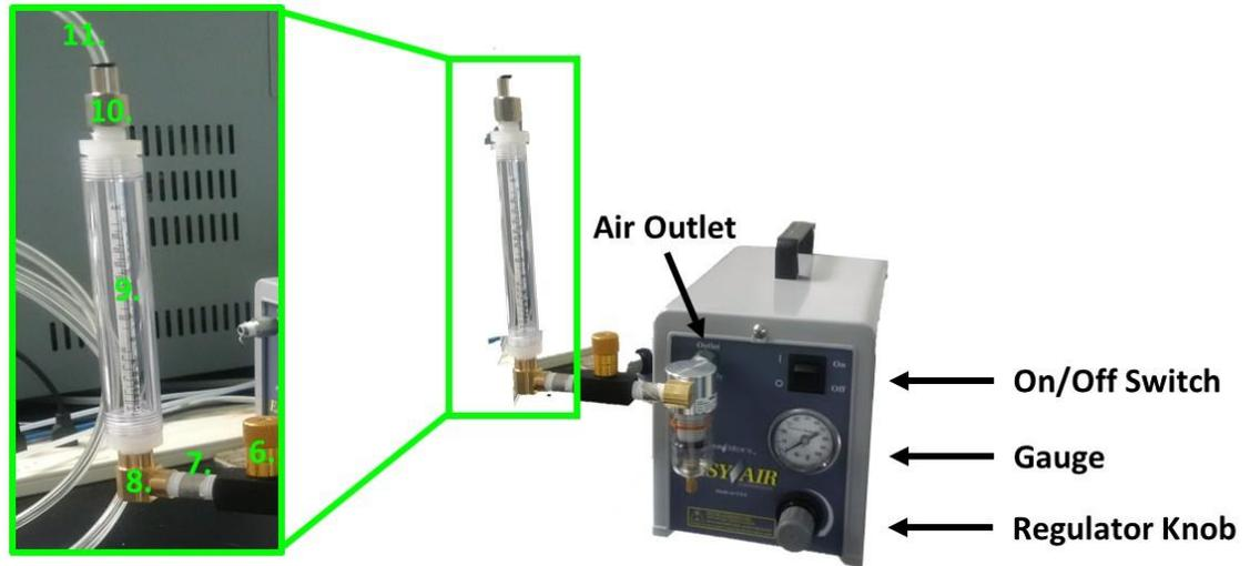
6. Easy-Set threaded precision flow-adjustment valve (McMaster-Carr 46425K22)
