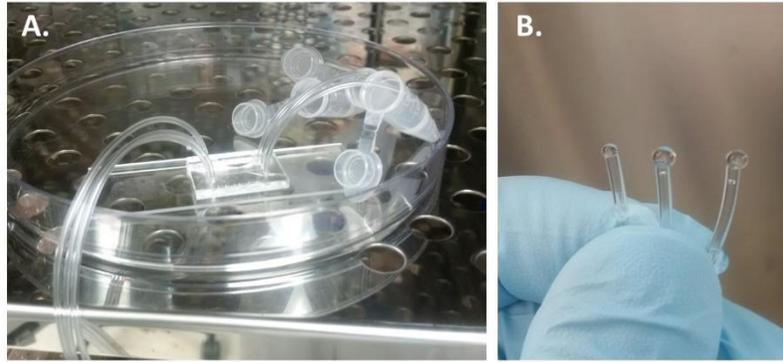
**Figure 3.** To capture the media leaving the device during a media change, 1.5-ml microcentrifuge tubes can be used as waste reservoirs (A). (B) Use the infuse arrow on the syringe pump to advance media until a droplet forms at the top. If any air bubbles are observed in the tubing, continue to advance the media to push out the air bubbles.
