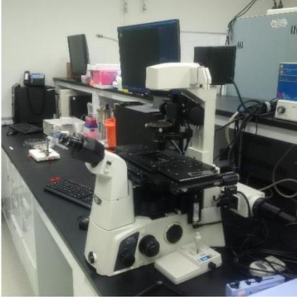
An inverted microscope is used to examine the devices for trapped air, as well as for live imaging when the devices are being seeded with cells. Microscopes with a fluorescence capability can aid in imaging the devices after staining with fluorescent dyes or conjugated antibodies.
