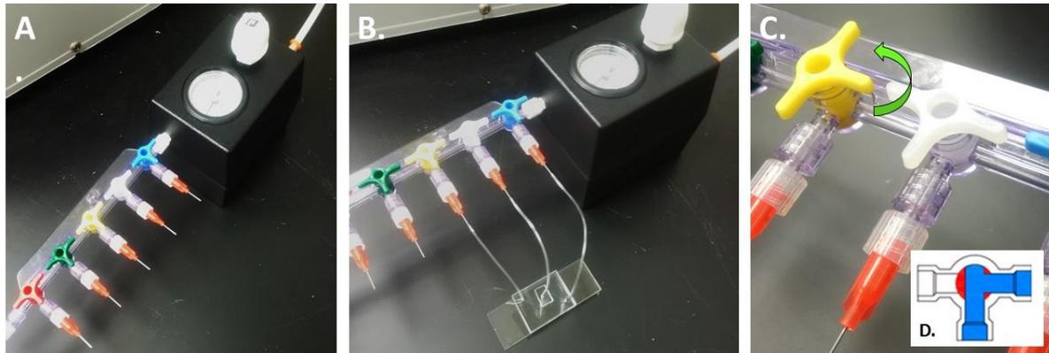
**Figure 6.** The Multiple Port Manifold is connected to a Pneumatic Primer (A). All 3 ports of a microvascular network device with a 3D tissue chamber are connected to the manifold (B). (C) Turn the 3-way valve counterclockwise on the T port, so that the flow of gas is directed into the last port of the device (D; inset graphic from <https://valveman.com/blog/understanding-tport-vs-lport-directional-flows/>).
