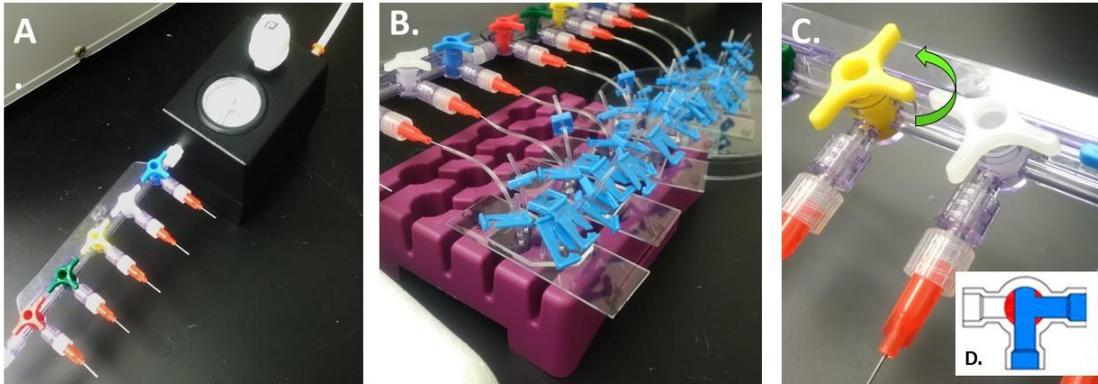
**Figure 6.** The Multiple Port Manifold is connected to a Pneumatic Primer (A). Multiple SynVivo devices are connected to the manifold (B). (C) Turn the 3-way valve counterclockwise on the T port, so that the flow of gas is directed into the last port of the device (D; inset graphic from <https://valveman.com/blog/understanding-tport-vs-lport-directional-flows/>).
