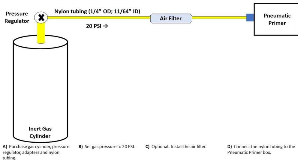
**Figure 4.** Schematic for connecting the Pneumatic Primer to a source of inert gas.
