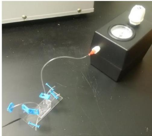
**Figure 5.** Schematic for connecting the microfluidics device to the Pneumatic Primer.
