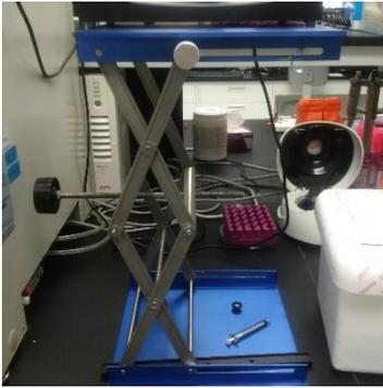
A lab jack with 12-inch x 12-inch plate (30.48 cm x 30.48 cm; Fisher Scientific S63083) is used to safely elevate the syringe pump beside a tissue culture incubator. The syringe pump should be higher than the shelf with the microfluidics device, so that fluid is not being flowed uphill against gravity.
