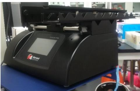
A syringe pump (PhD Ultra is shown; Harvard Apparatus; SynVivo 301001 or 301002) is used to maintain media flow to cells inside the devices. A multi-syringe rack can provide space for multiple syringes and increase the number of microfluidics devices receiving media at one time.
