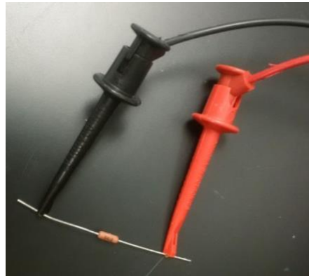
Figure 7. Connecting the test leads to the calibration test resistor.
