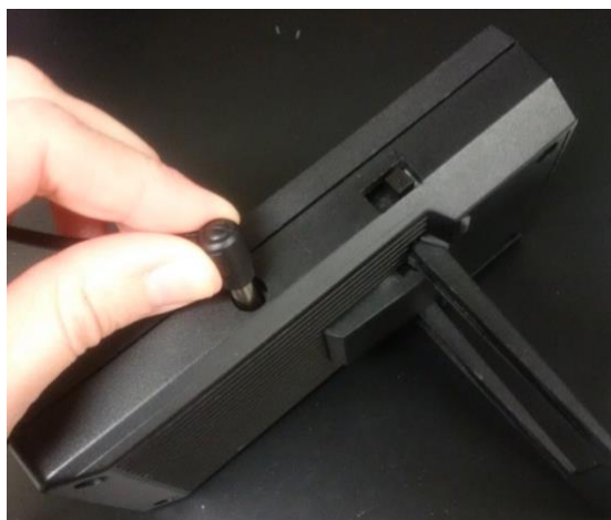
Figure 3. Connecting the power cable to the Cell Impedance Analyzer.
