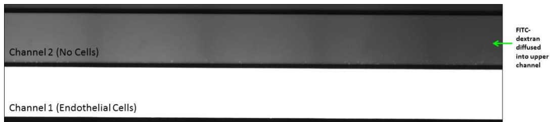
Figure 3. Fluorescence image of a permeability assay captured after a 1-hour infusion of 4 kDa FITC-dextran.
