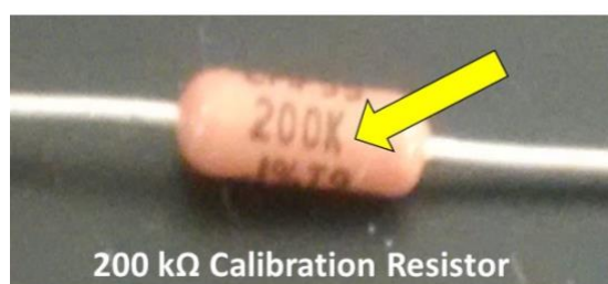
Figure 6. Reading the value and tolerance on the calibration test resistor. The value of the resistor is highlighted with a yellow arrow. This resistor is marked “200K”, indicating a resistor value of 200 k \Omega .
