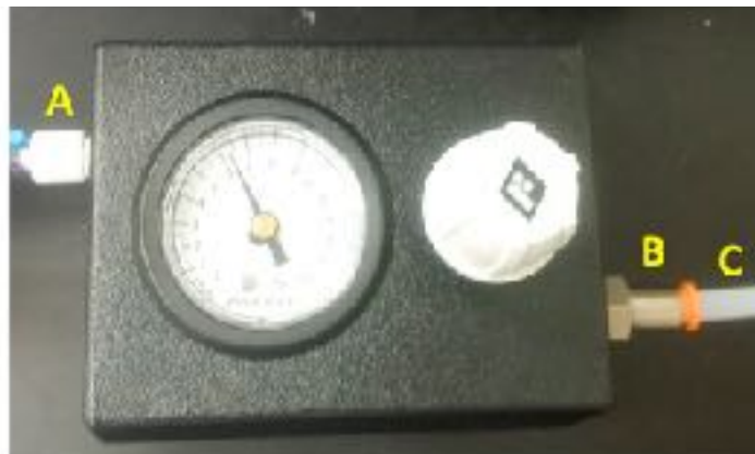
Figure 1. A top view of the Pneumatic Primer, containing an inlet connector for the device (A), a metal male connector to the gas line (B), and nylon tubing that connects to the gas tank (C).
